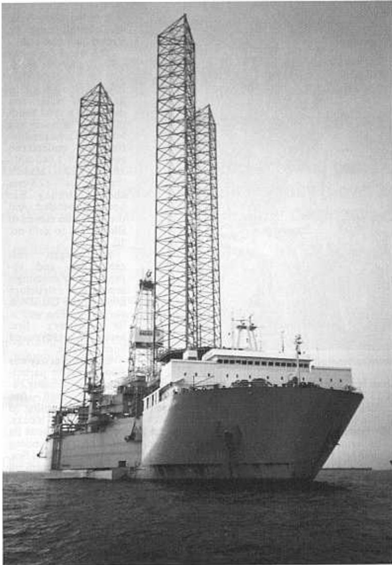
Once the Santa Fe Galaxy I jackup was loaded on the deck of the transport vessel (left), seafastening operations began in preparation for the long voyage to the North Sea. To ensure the initial stability of the vessel with her cargo, large, custom-built sponsons (right) were used.
